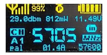
Note : The RF power information on OLED display is PA chip detector power , not is actual RF output power
