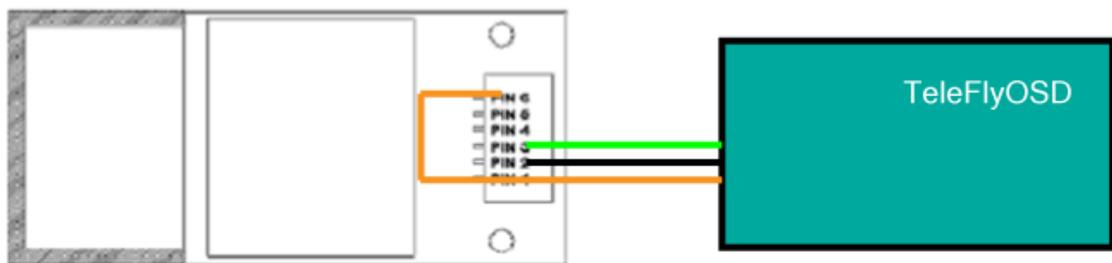
**CAUTION: GPS PIN#1 and PIN#6 MUST be connected to +3.3V. This GPS doesn't work without PIN#6 connecting to VCC.**
