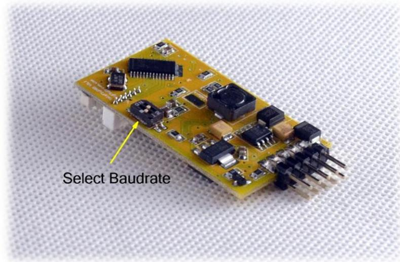
The arrow-indicated DIP switch in the figure has an ON mark above. There may be four different baudrate combinations via setting of this switch:
