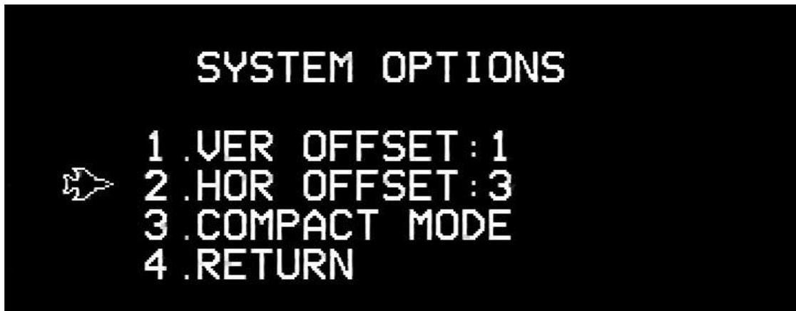
To change options, use the "UP" and "DOWN" buttons to move the marker to the appropriate option and press the "SET" button.
