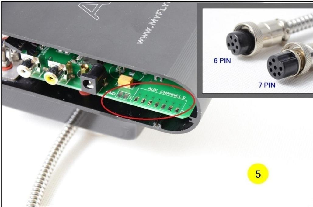
After removing the left panel you will see there are 7 soldering pad on the PCB. They are numbered from 1 to 7.
