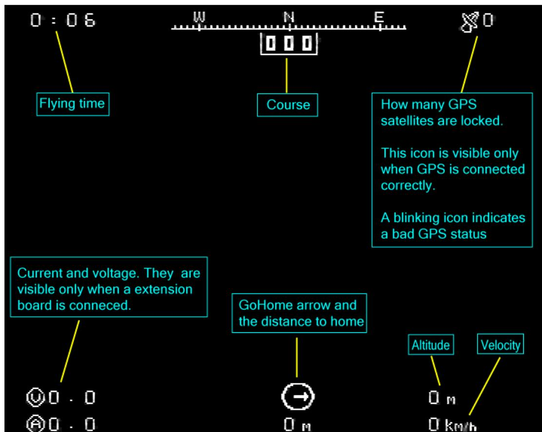
The reading meaning of various parts in the picture has been marked.
