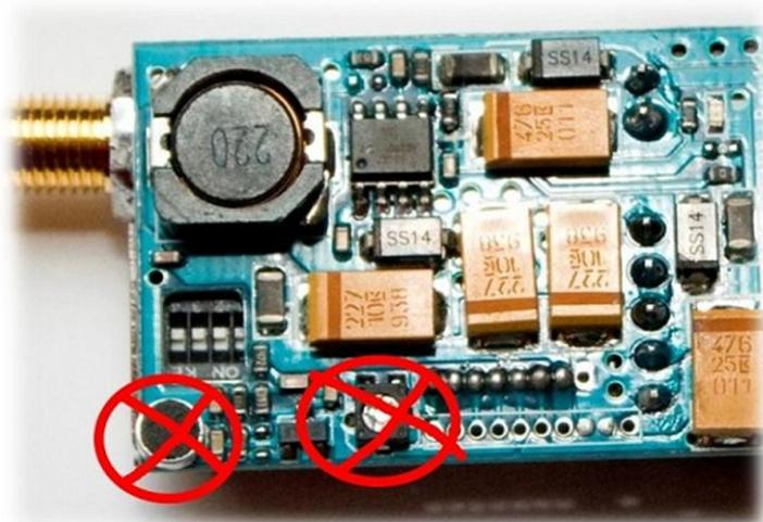
The microphone and potentiometer in the red circles must be removed to get a clean audio channel.
