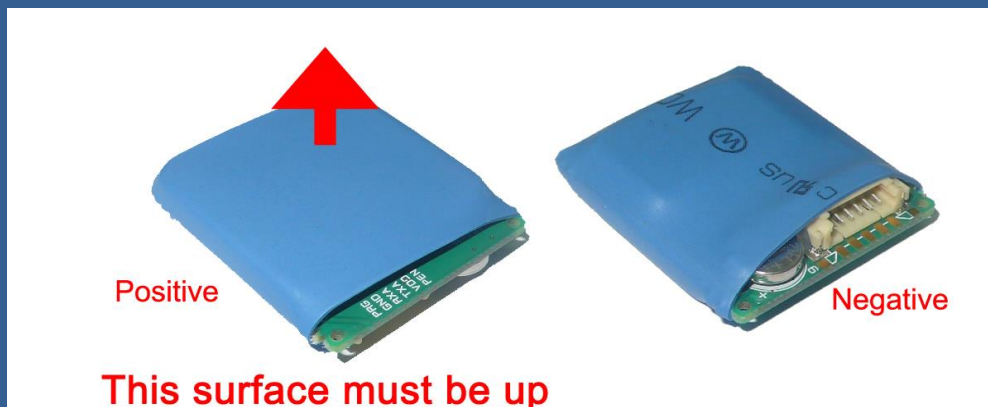
GPS Module Installation
